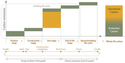
Figure 4: Scope of carbon emissions across different stages of the building life cycle
