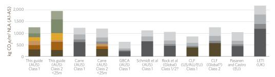
Figure 15: International residential (Class 1 & 2) embodied carbon benchmark (Average practice) Sources: The Footprint Company<sup>48</sup> Carre<sup>50</sup> GBCA<sup>51</sup> Schmidt et al.<sup>52</sup> Röck et al.<sup>53</sup> CLF<sup>21</sup>, Pasanen and Castro<sup>54</sup> and LETI<sup>20</sup>
